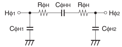
Horizontal transfer clock equivalent circuit
