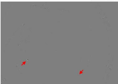
The pudding cup's top film would normally be challenging to inspect for pinholes. The film's glossy, undulating surface reflects light in arbitrary directions, producing random reflections. Furthermore, the surface contains printed graphics, making it difficult to differentiate between dark print and a pinhole.
