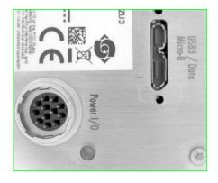
The Hypel imaging system acquires multiple images of an object, each captured using a different camera exposure duration. The brightest image reveals details inside of the electrical connectors, but other areas are lost in the saturated pixels. The darker images better capture the label content and brushed aluminum surface, although the connector detail is lost. The resulting image (shown at bottom) delivers detail of all object features.
