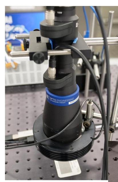
An object, such as that shown below, may have features on several planes. Or, the distance between the lens and the object may vary. When imaged under magnification, it is often impossible to capture an image having sharp focus. Simply put, the laws of physics get in the way.
