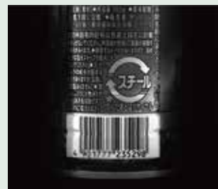
Light: IFHA-150W (LWD=10mm) The effect of reflections is small even on a curved surface, and the recognizable area is wide.
