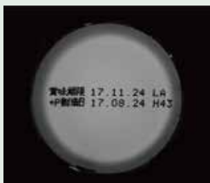
Ring light: IMAR-130DW (LWD=60mm) Shadows are reflected around the printed area that make it difficult to recognize characters.
