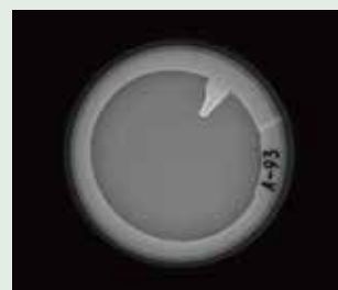
Light: IFHA-150IR-850 (LWD=15mm) Infrared can erase printing other than printed letters, and can recognize the printed area in addition to scratches, contamination, etc.
