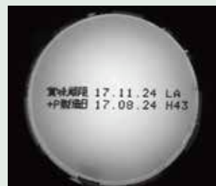
Light: IFHA-150W (LWD=10mm) Characters can be easily recognized due to low shadow reflection.
