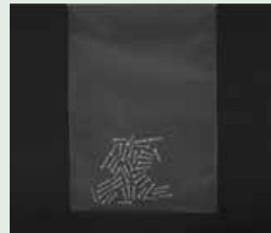
Light: IFHA-150W (LWD=10mm) The surface halation is reduced and internal quantity can be easily inspected.
