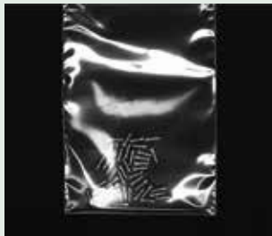
Ring light: IMAR-130DW (LWD=100mm) Halation occurs on the surface of the bag and is not ideal for quantity inspection in the plastic bag.
