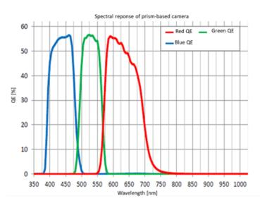
Fig. 6 - Spectral separation of a prism-based camera with IR-cut filter
