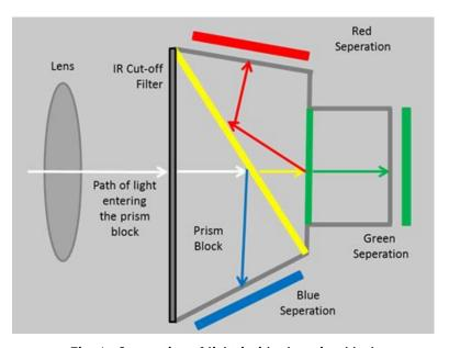
Fig. 1 - Separation of light inside the prism block
