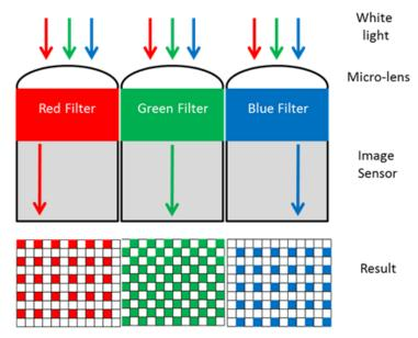
Fig. 2 - Filtering of light on a Bayer sensor
