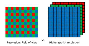
Fig. 9 - Bayer RGB vs multi-sensor camera resolution
