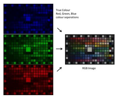
Fig. 3 - True color imaging with multi-sensor prism cameras
