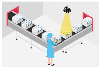
Counting objects in a package for completeness can save you from an unsatisfied customer. For example, one shoe is not sufficient, three shoes are too many. For handy sized objects the blaze camera delivers perfect data to count them, independent of color and contrast. No additional light source is needed.
