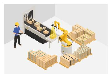
Next day delivery and mixed pallets require fast and versatile robots to stake any article tightly onto a pallet. Therefore, machine vision is required to guide the robot. The camera data is used to determine the shape, position and orientation of the pickable object and to find its best lifting point. Robustness, compact size and light weight allow its assembly on the robot arm.
