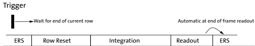
Figure 37: Entering and Leaving a Global Reset Sequence
