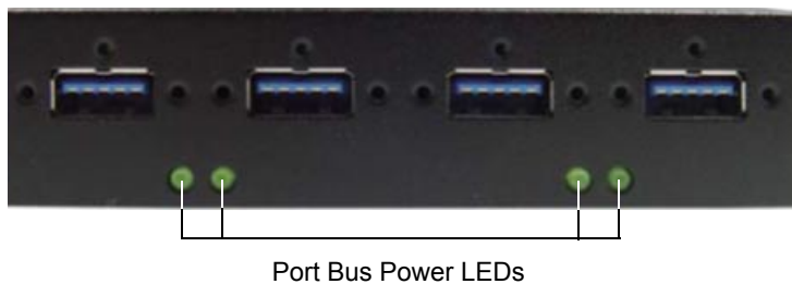
Fig. 4: Rear of the Hub
